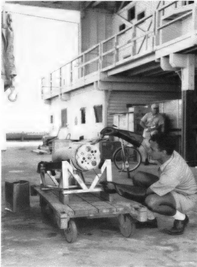
FIGURE 9-23. TEAK INSTRUMENTATION POD SHOWING RADIATION EXPERIMENTS
